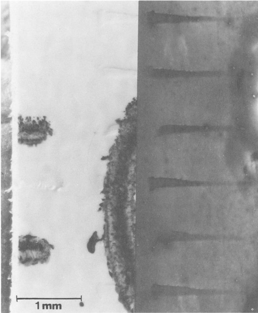
FIG. 9—Comparison of drive wheel impressions on test tapes with and without manufacturer's printing and marking pen enhancement.
